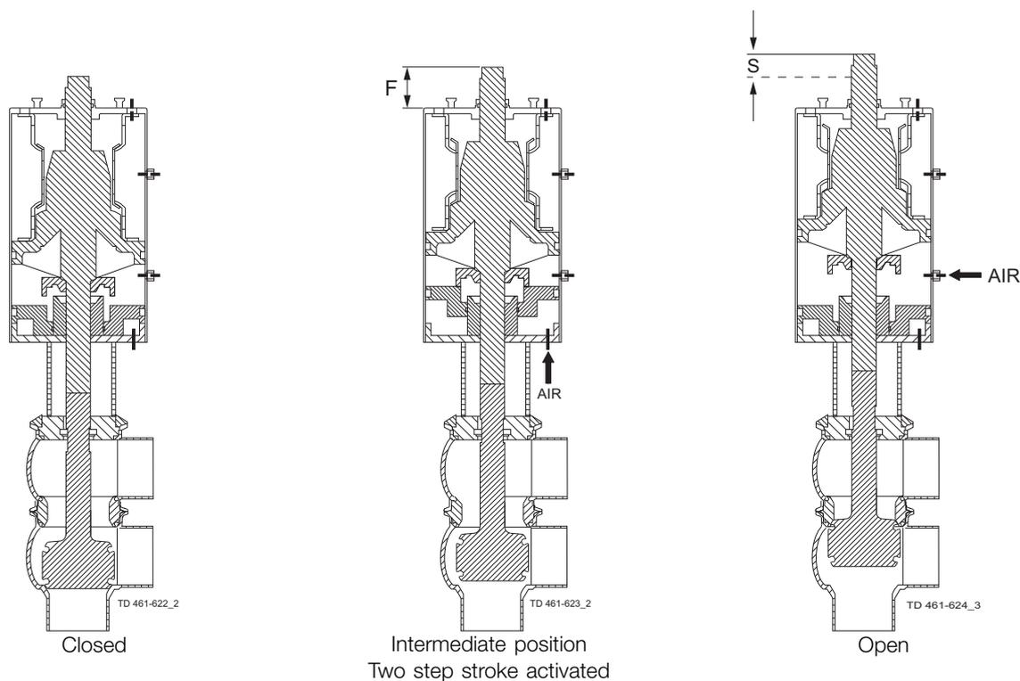
The plug opening for different change-over valves and actuator size is shown below.
