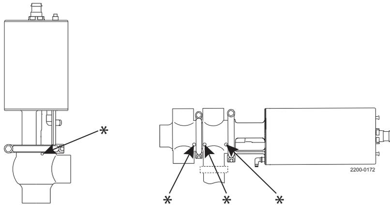
\* = Leakage detection hole
