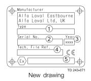
In addition to the standard pump nameplate, ATEX Certified units have an additional ATEX name plate affixed to the pump gearbox housing stating the unit ATEX certification standard. Name plate example:
